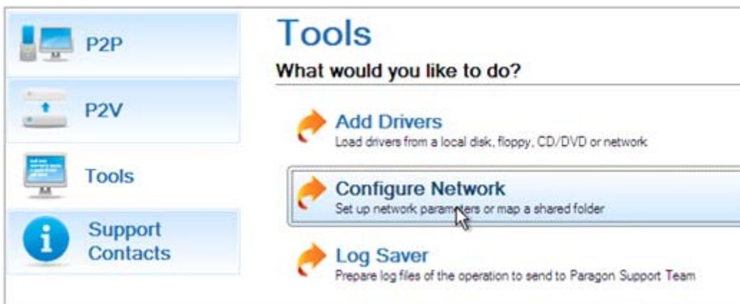
2. In the opened dialog provide an IP address, a network mask, default gateway, etc. for your network device.
